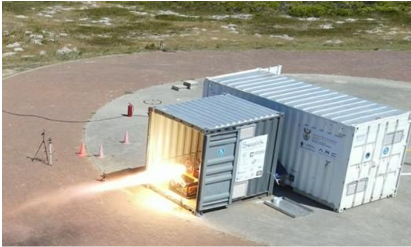
Mobile Propulsion Test Facility
