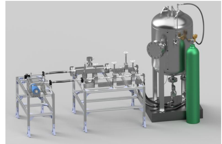
Propellant Pump Test Facility
