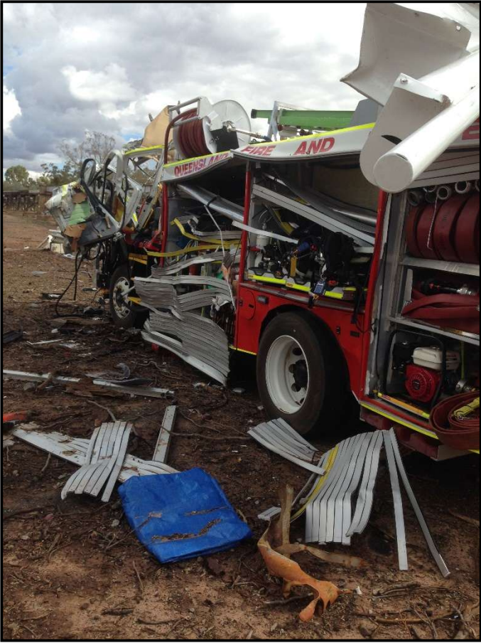
Picture 19 – Rear view of damage to fire engine from blast
