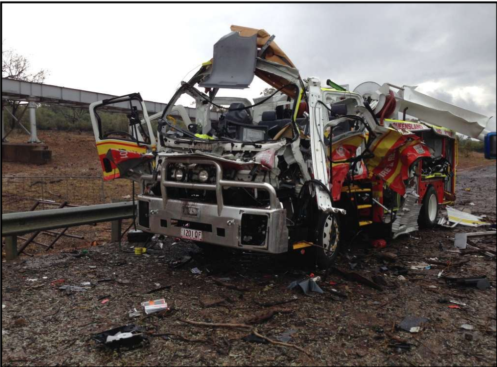
Picture 18 – Frontal view of damage to fire engine from blast
