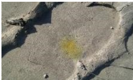
Above: Greenish colouring on soil (non explosive) flamed by means of gas lance
