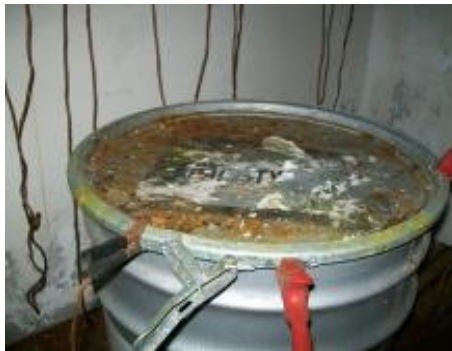
Dried out lead styphnate tarnishing on drums
