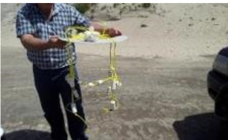
Above: A mask consisting of detonating cord and RDX pellets was designed to assist with the placement of the charge over the drum from a distance making effective use of explosive force.
