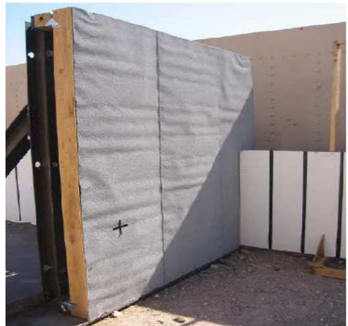
Figure 2: Panelized plywood target
