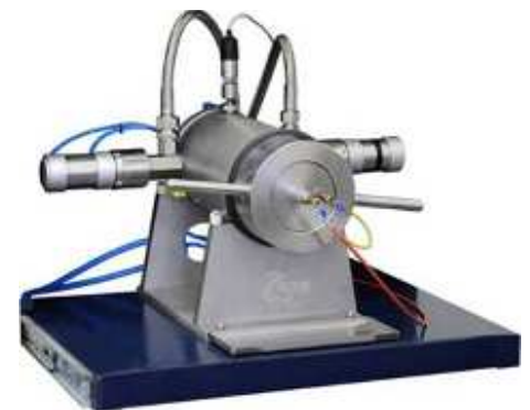
Figure 3 (below): Stojan vessel (top) and example plots of typical raw record pressure (MPa) vs. time (centre) and the resulting burning rate (m.s -1 ) vs. pressure dependency (bottom) obtained from just one shot.
