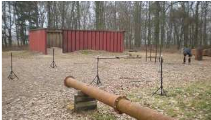
Figure 6: Detonation chamber (left), test polygon with blast wave sensors being set up (right)
