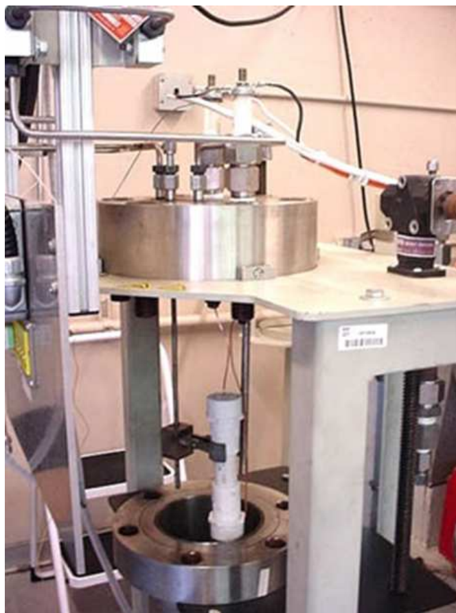
Figure 5: Minimum Deflagration Pressure – Bomb and internal assembly to hold cylinder of test explosive. Photograph courtesy of Natural Resources Canada (CERL)
