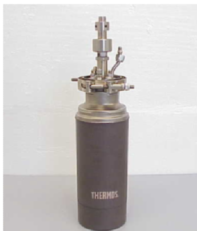
Figure 4: Adiabatic Dewar calorimetry with SS Dewar. Control and measurement system illustrated. Photograph courtesy of Natural Resources Canada (CERL)
