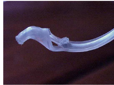
Figure 3: Example of tube tip that was partially melted and ignited
