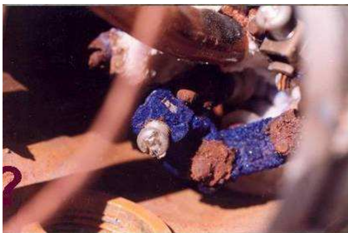
Figure 2 (Above): Crystals of tetramine copper (II) nitrate formed by the interaction of AN with copper in an electrical box on an explosives plant.
