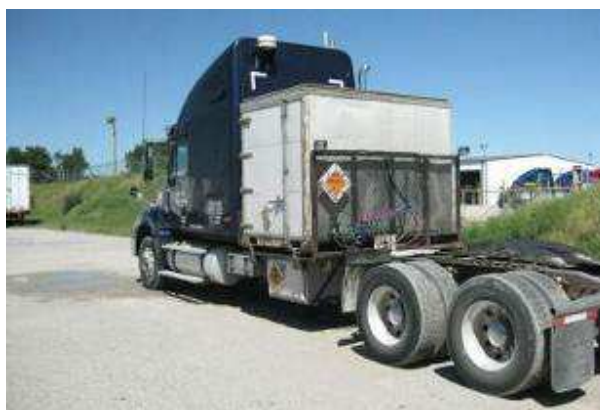
A second transport vehicle offers additional segregation alternatives
