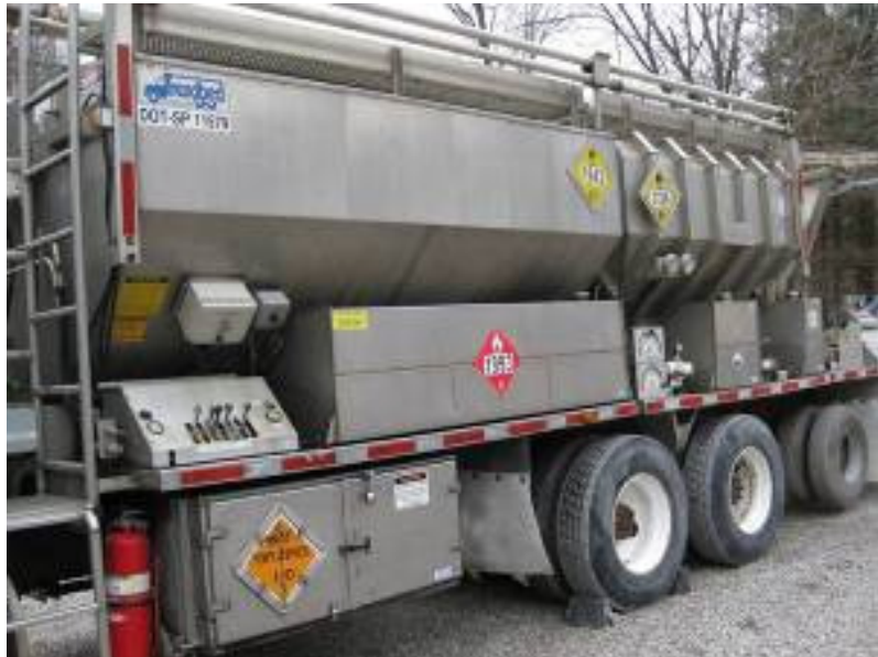
Figure 1: Multi-purpose bulk truck
