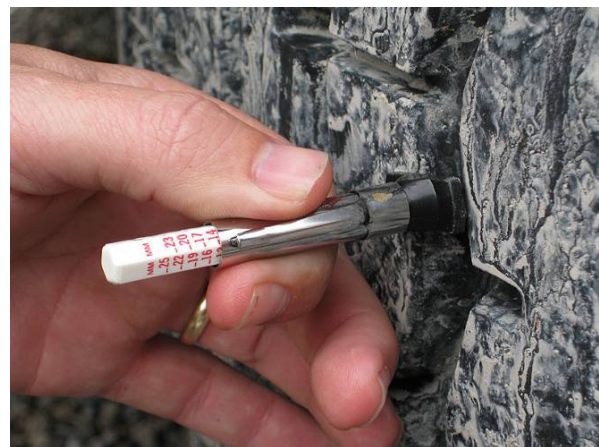
Figure 3: Checking tread depth across width of the tyre.
