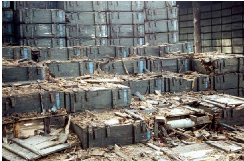
The photograph shows a deteriorating open-air AXO dump. Since these munitions were temperature-cycled over a long time, they cannot be cleared by moving, but should be detonated in situ . (Photo courtesy OSSE)
