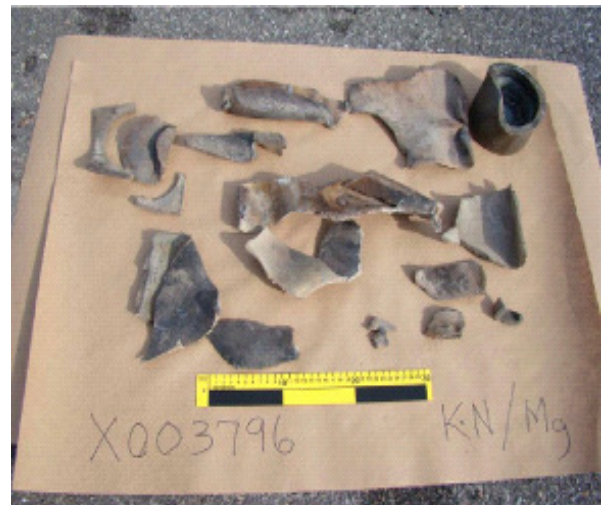
Figure 2: Fragments produced from a pipe bomb containing a potassium-nitrate based homemade explosives.
