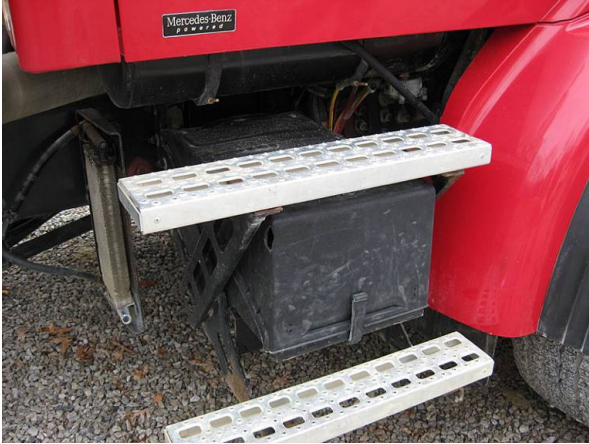
Figure 4: Battery housing protected by the step
