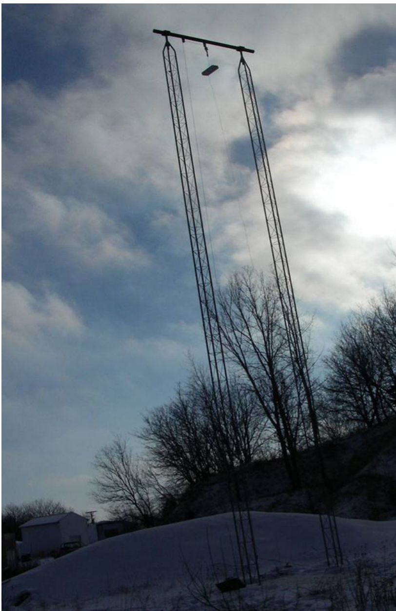
UN 12m drop test: If there is an ignition, the product is forbidden for transport.
