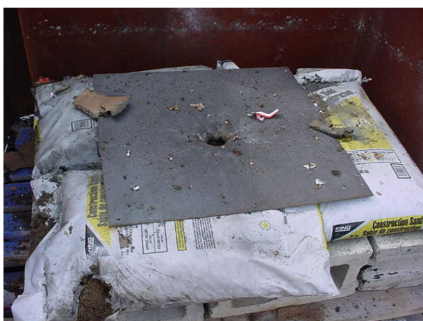
Figure 2. Damage to witness plate following the testing of a package of perforating charges, each with a with net explosive quantity of 19 g
