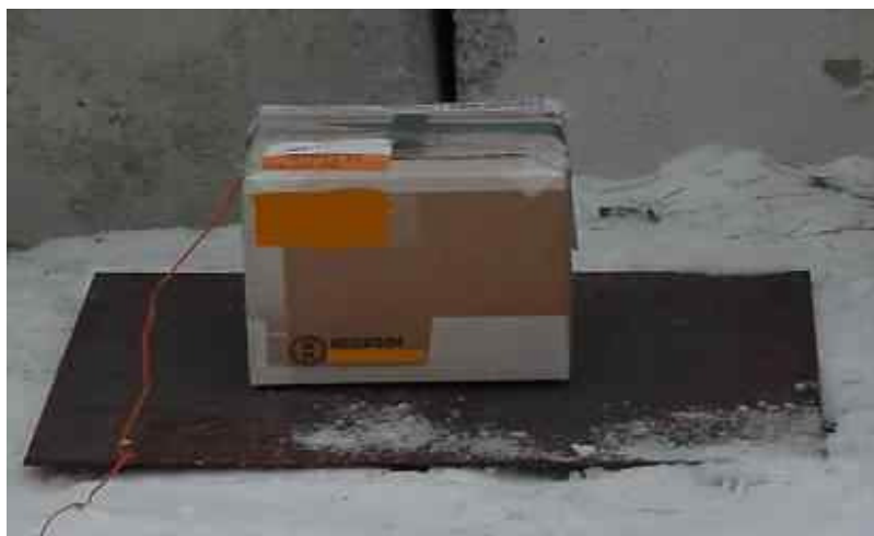
Figure 1. Example of the experimental setup for the 6(d) test at CERL. The white material on the ground is a very effective Canadian solution for reducing the probability of grass fires!
