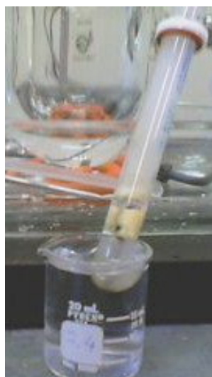
Figure 1b: pH/T probe new and after high temperature cycling abuse.
