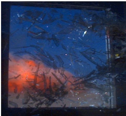
Figure 2. Glass shards from an unprotected window
