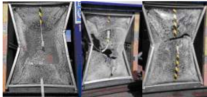
Figure 8. Anchored film response under high blast loads
