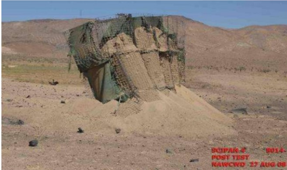
Figure 19: Barricade Remains—Post Detonation
