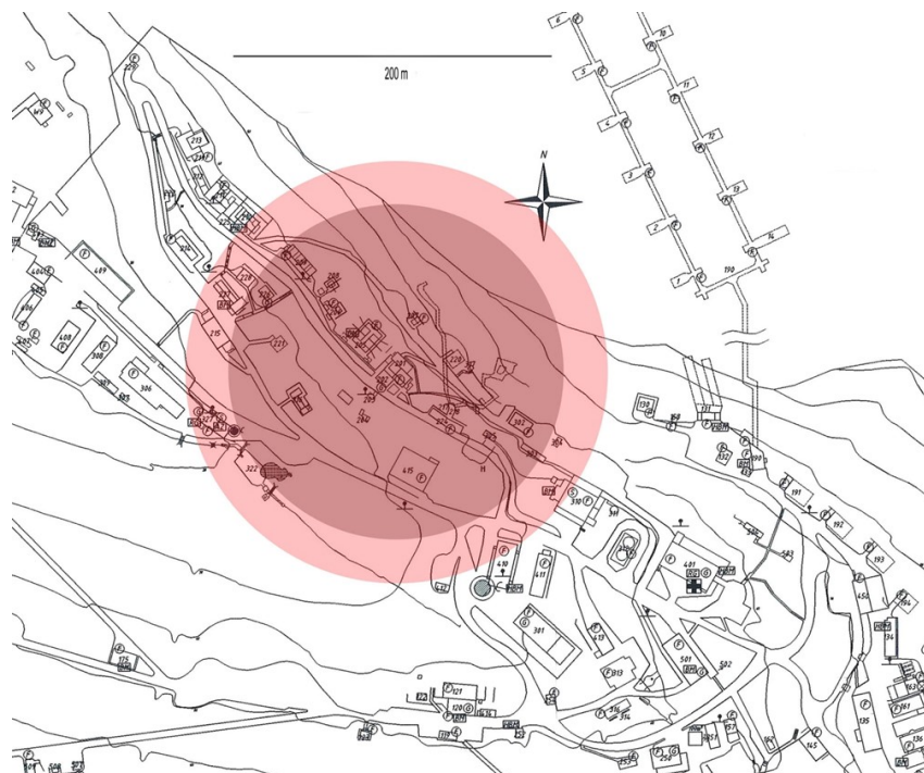
Figure 3 – Safety zone for blasting the effluent barrels (dark red: safety zone calculated for 100 kg of explosive, light red: calculated for 200 kg of explosive)
