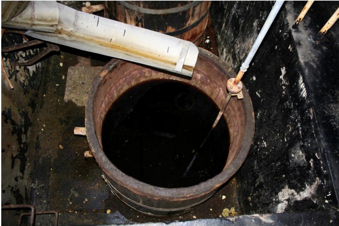
Figure 1 – Wooden effluent barrels containing metallic iron shavings and Sulphuric Acid
