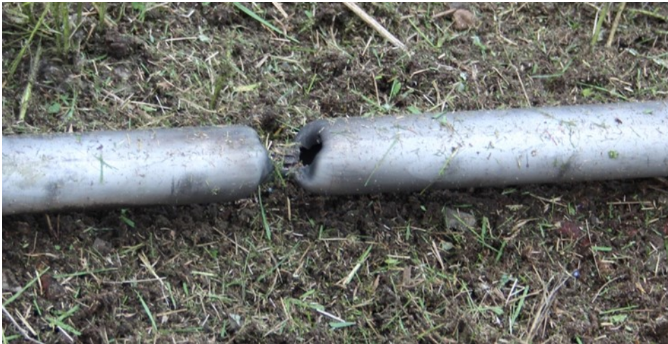
Figure 27 – Cut steel pipe after blasting with detonating cord
