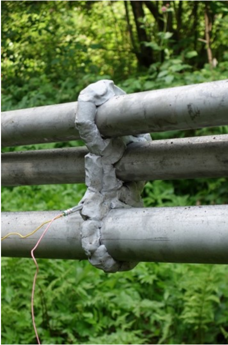
Figure 28 and Figure 29 – Emulsion explosive charge applied on steel pipes
