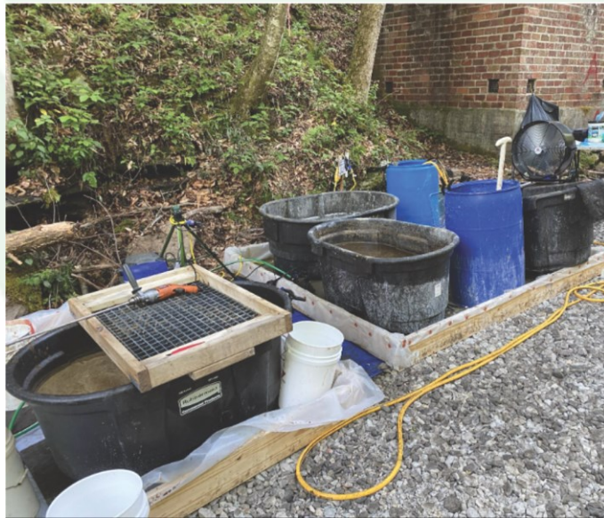
Destruction of Dynamite in MuniRem Reagent Solution
