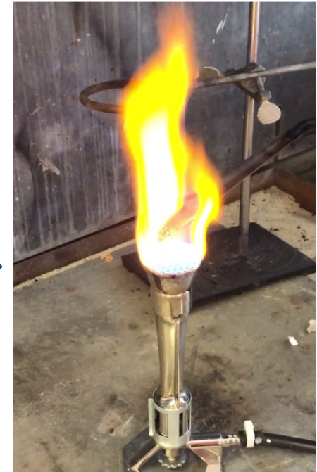
Lead Styphnate post MuniRem Treatment – Zero activity in an open flame
