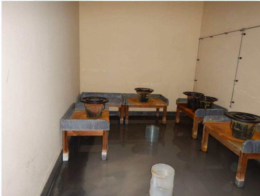
Magazine Interior with poorly stored primary explosives
