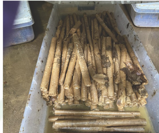
Recovered Dynamite in Plastic Tub and Soaked in MuniRem Solution
