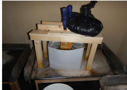
Figure 1. Plastic cups in a storage magazine, each holding 0.5 kg of tetrazene. Aqueous solution of MuniRem was sprayed to render safe areas around the containers (left), and a customized soaking system to neutralize the explosives in the storage cups to enable safe recovery (right) were installed.
