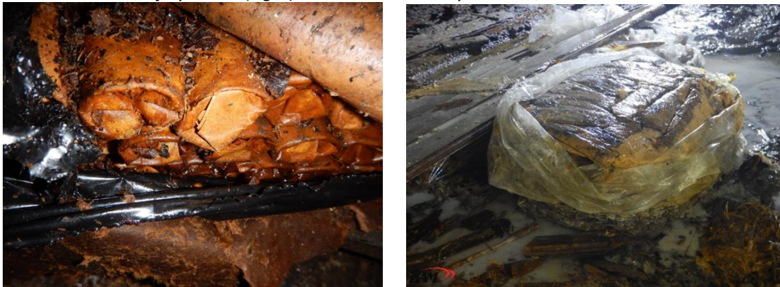
Figure 7. Sweating dynamite without (left) and with a solution of MuniRem reagent applied (right) to neutralize and destroy the nitroglycerin. Photos are courtesy Ram Inc, Ohio, USA
