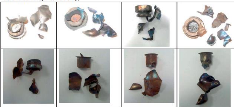
Figure 5. Examples of tube deformation and fragments in MTC6.
