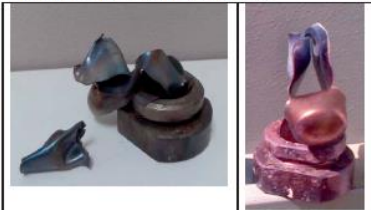
Figure 4. Tube deformation and fragmentation patterns reproduced from Koenen and Ide's 1956 papers
