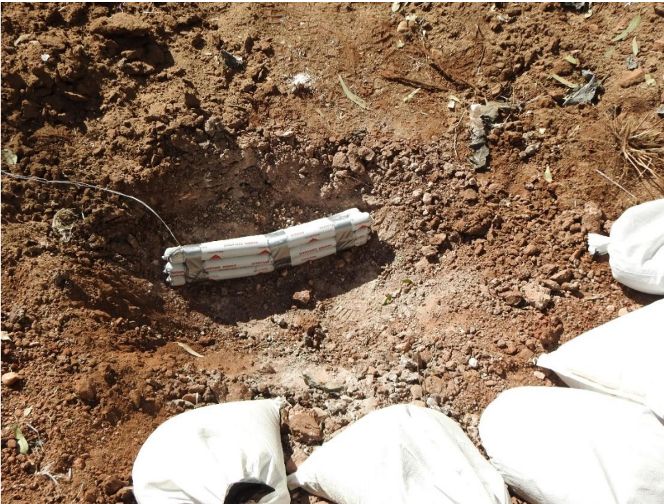
Figure 13: Crater of first bomb after cleaning out the broken ground. Pulverised white deposit in the soil is evident. Apparent diameter \approx 1\text{m} .
