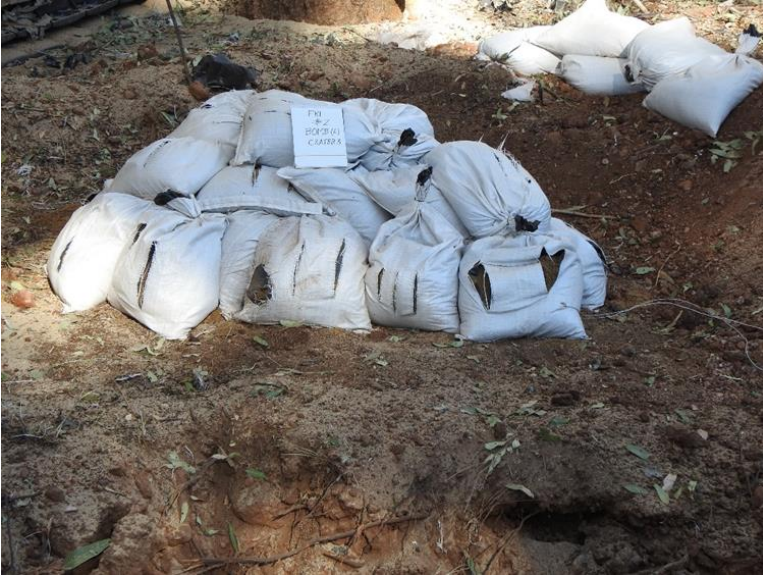
Figure 12: Dome of sandbags placed over 5kg charge to suppress blast noise
