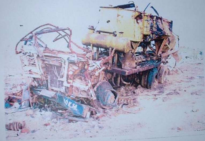
RECL DAMAGED BMD SYSTEM LOADED WITH NON EXP MATRIX VEH NO. UP 65 1565 PARKED NEAR AN STORE
