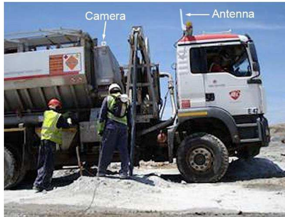
(Above) MMU showing the WiFi antenna of Blast- i TM system. The GPS antenna is on the other side of the vehicle cab.
