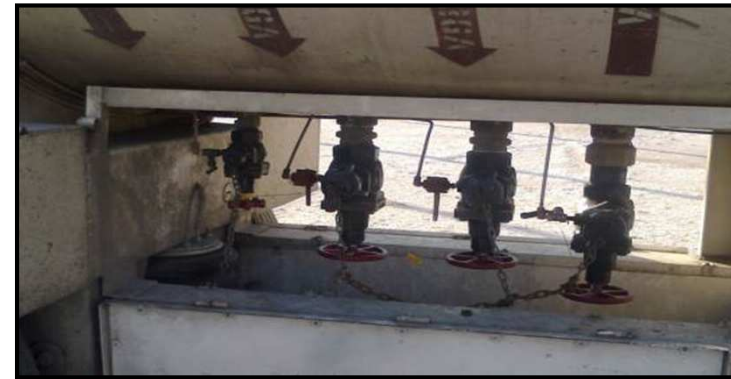
Picture 2: Tank trailer discharge valves (one for each chamber)
