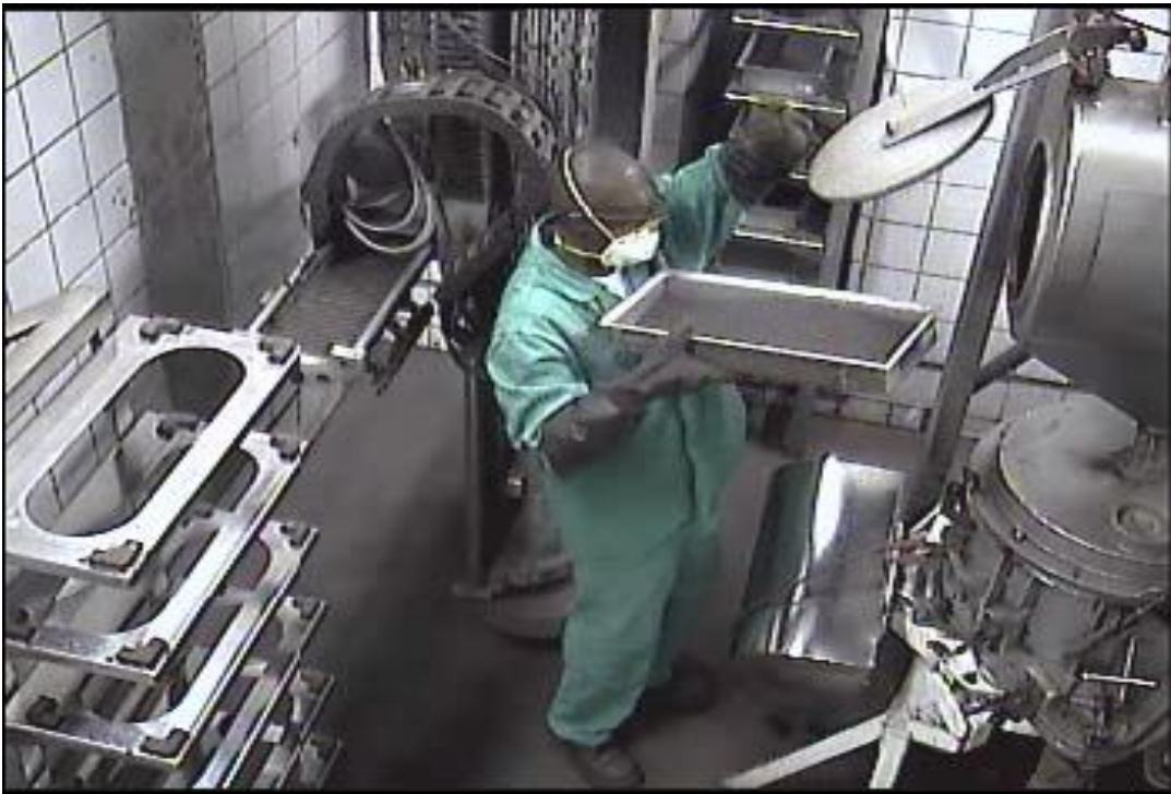
Employee tried to insert tray of G composition into auto tipper but lost his grip on the tipper hatch which began to fall under gravity.
