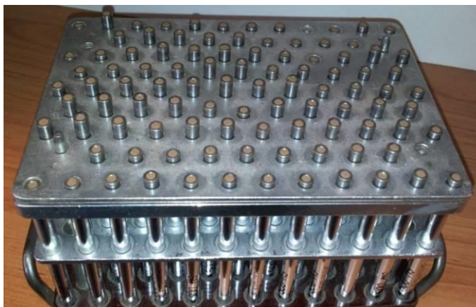
Figure 1: Delay elements before pressing into shells
