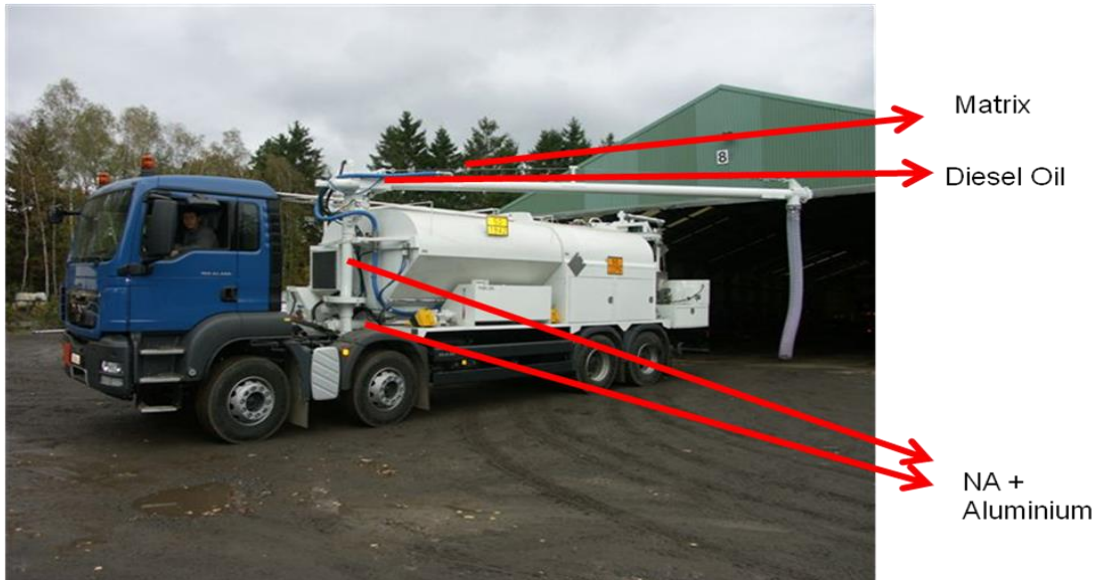
Picture 1 : EPC-Belgium –Multiblend truck (Tradestar unit)
