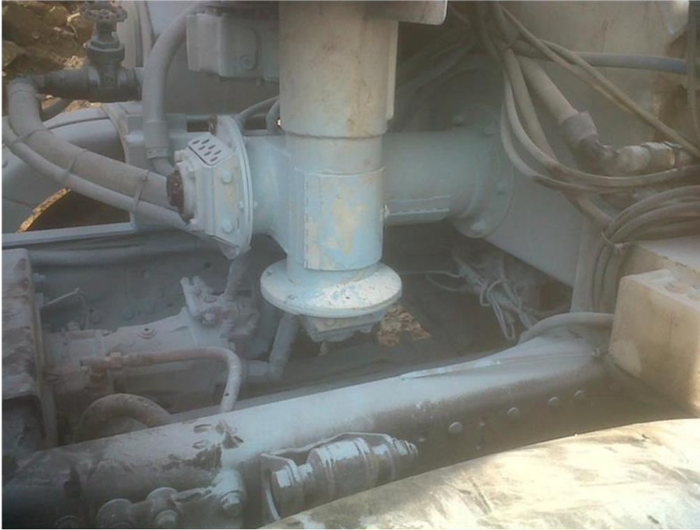
Picture n°2 : vertical auger with the bearing after the use of the extinguisher
