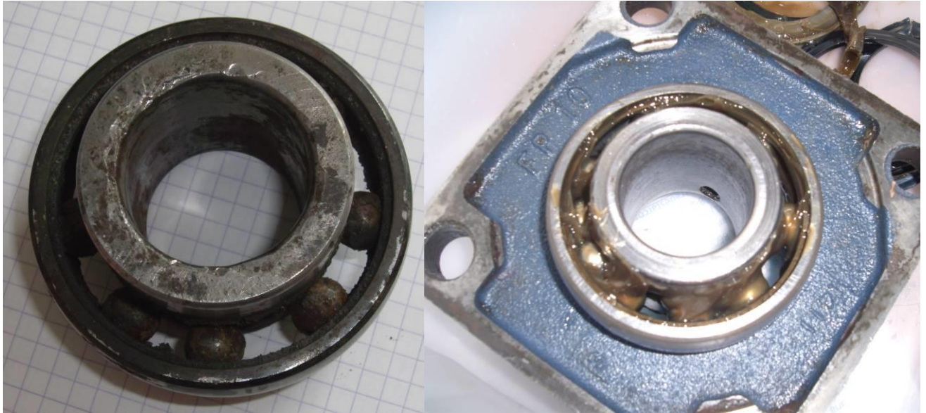
Picture n°4: ball bearing after the incident and a new ball bearing
