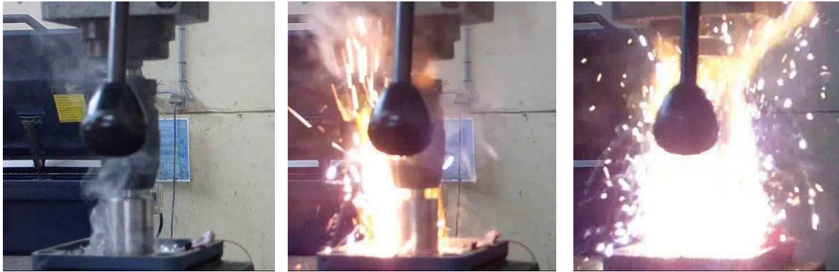
Pictures 6-7-8: reproduction of the fire in the lab – bearing SKF
