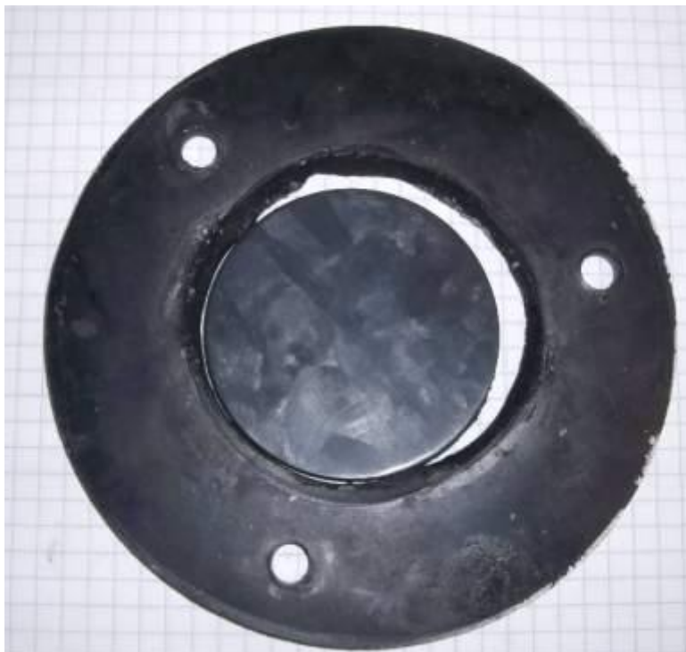
Picture n°3 : gasket seal deformed (inside circle with the diameter of the shaft)
