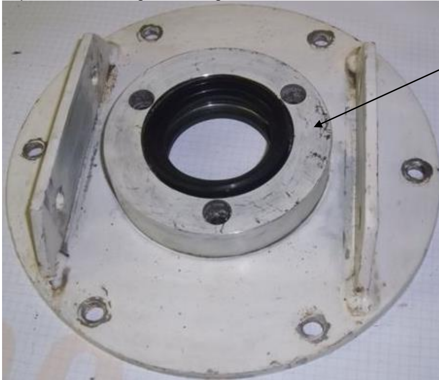
Picture 9 : Additional element to improve the sealing of the auger.
