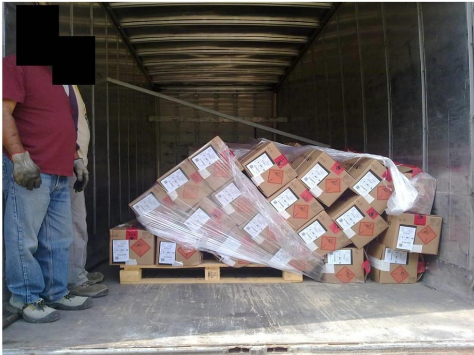
Figure 1: the explosive overturned at the warehouse of destination
