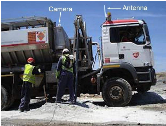
Figure 6: An MMU showing the WiFi antenna of Blast- i ™ system. The GPS antenna is on the other side of the vehicle cab.
