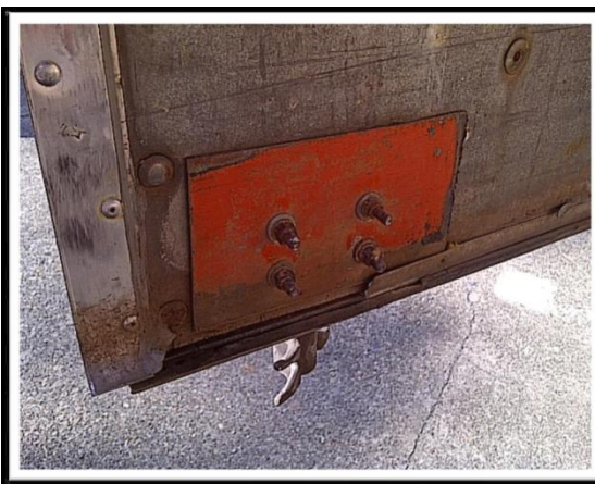
Picture 7: Repaired door and protruding screws
