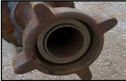
Picture 3: Hose coupling
