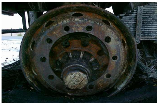
Rim / Brake drum assembly of the missing wheel
