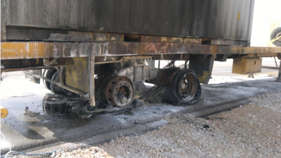
Figure 5a: Condition of the rear right axle after the fire
