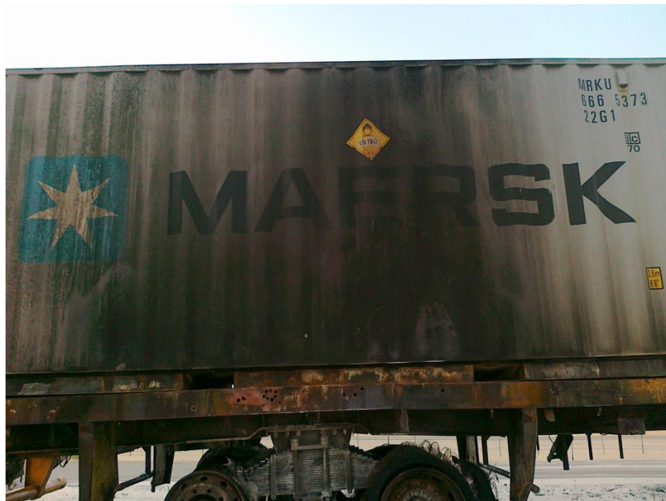
Figure 4b: Condition of the container after fire extinguishing
