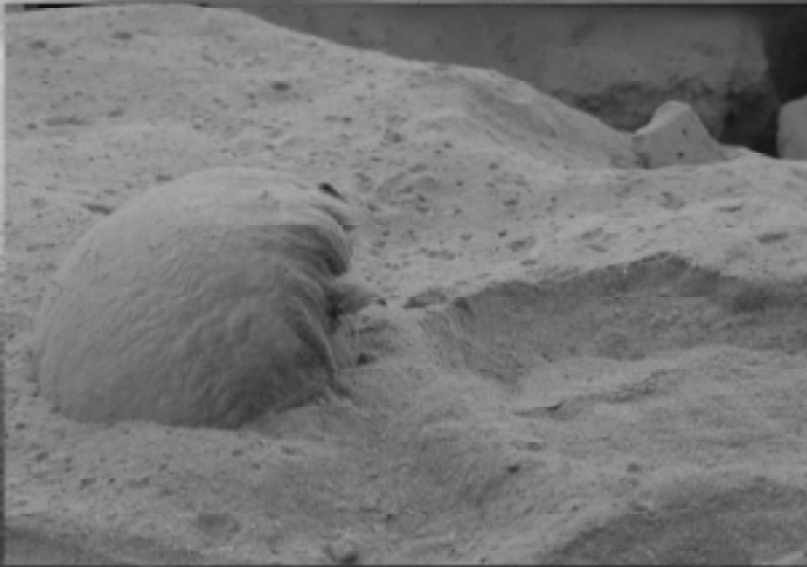
Lead block condition after blast
