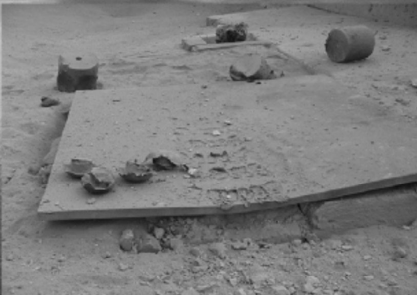
Steel plate base condition after blast
