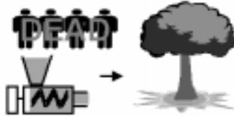
Contaminated emulsion thermal explosion/ detonation - Russia (multiple fatalities).
